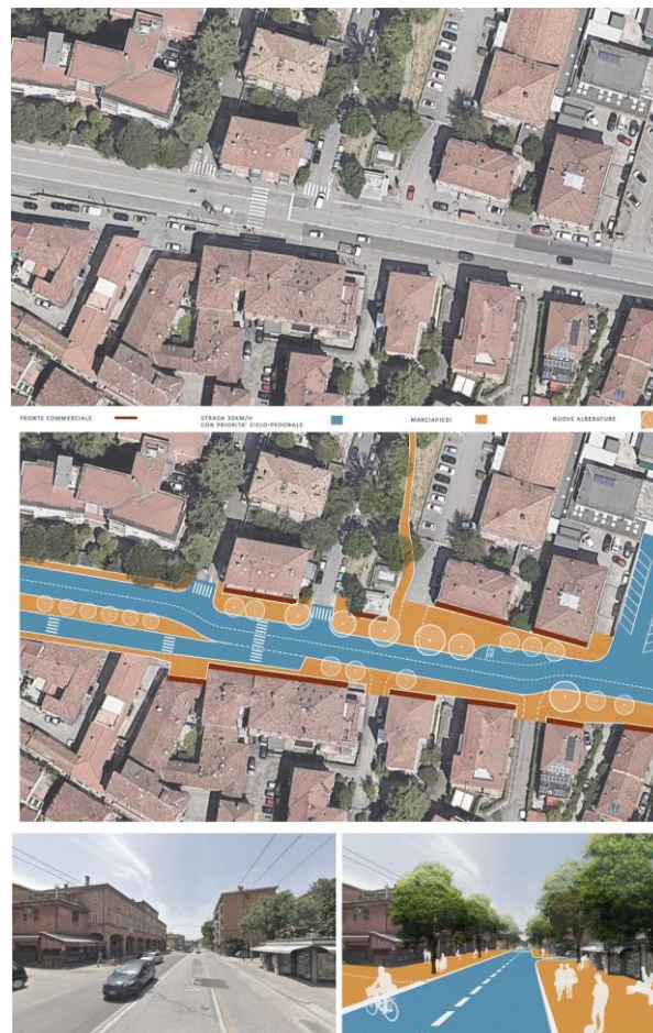
Figure 8. Interventions for improving the pedestrianization-motorization relationship proposed for the Massarenti area in Bologna (existing state and proposed arrangement plan of a section of Via Massarenti and view from below with existing state on the left and proposed arrangement on the right) (Developed by Authors)
