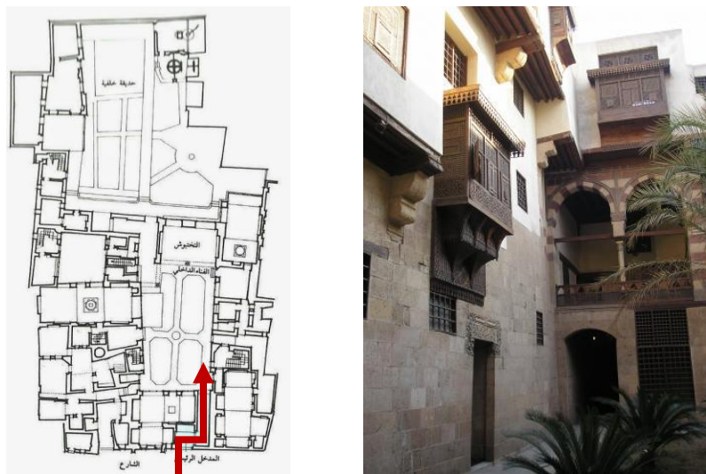
Figure 3. (a) Ground floor plan of Al Sehemy House (prototype of Islamic houses in Egypt) highlighting the Majaz at its main entrance, and showing the central rectangular court (Behrens-Abouseif, 1992), (b) Shot from the court of Al Sehemy house showing mashrabias on windows (Bayt Al-Suhaymi ("House of Suhaymi", n.d.)
