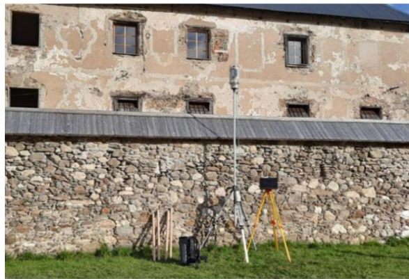
Figure 8. Scanning position "west façade"; the (remote-controlled) scanner is located about 10 m in front of the object at a height of 2.6 m; this does not obstruct the view
