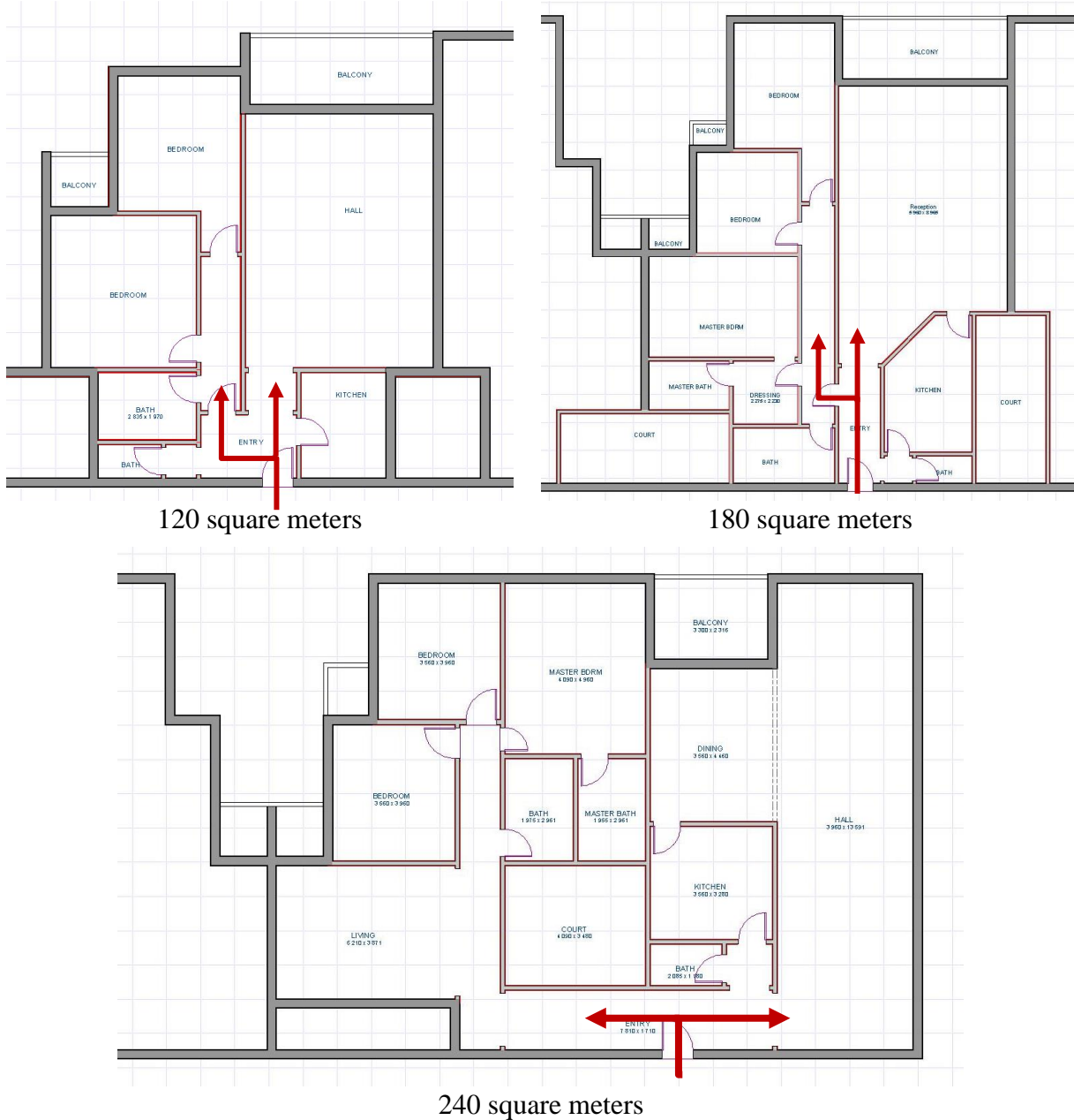
Figure 5. Proposed plans for residential units, having one elevation and various surface areas. All of them consider the appropriate zoning with different design (1 module equals 1 squared meter)
