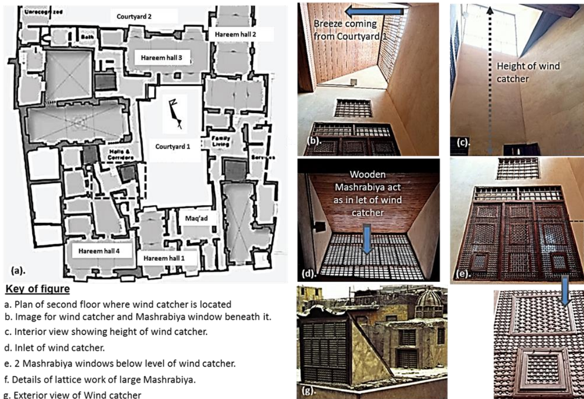
Figure 4. Integrated passive ventilation in hall 5 between wind catcher, courtyard1 and Mashrabiya in Bayt al Suhaymi: (Sources: (a) Abdelmonem, M. 2011, edited by author; (b – g) Developed by author)
